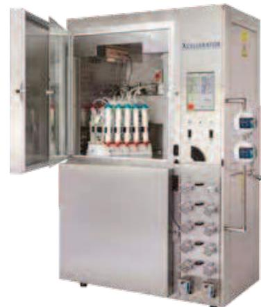
The XCELLERATOR supports two sizes of disposables. These options represent a 6x to 20x scale-up of the 160-mL bioreactor. The ten-bioreactor (ten 160-mL bioreactors) disposable is pictured above.
