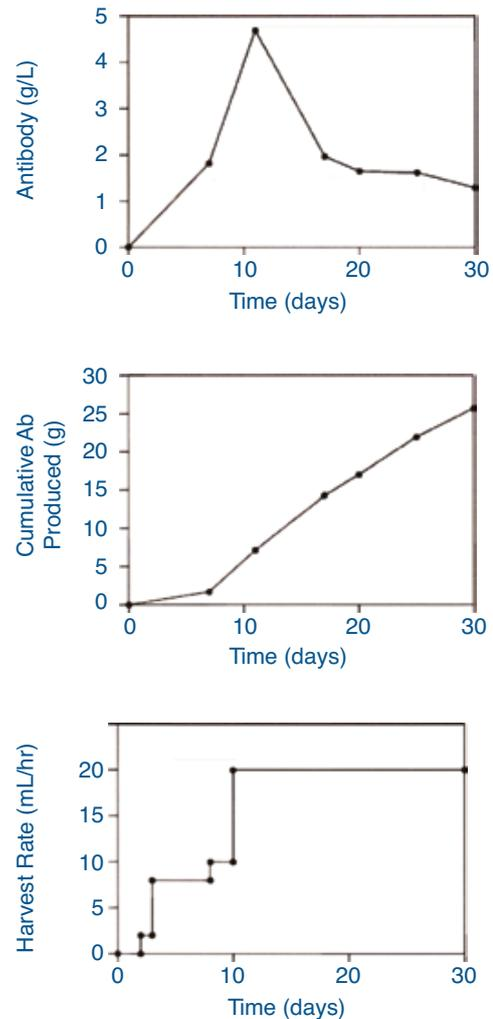
Figure 3: Antibody concentration, cumulative antibody production, and harvest rate from one 160-mL bioreactor
